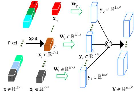
Fig. 4. An illustration of the proposed groupwise band convolution.  $\odot$  denotes the concatenation operation.
