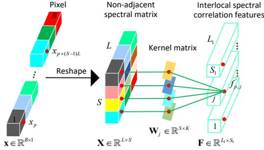
Fig. 3. A detail architecture of the proposed intergroup spectral extractor. The red solid-circles show the process of interlocal spectral correlation extraction.
