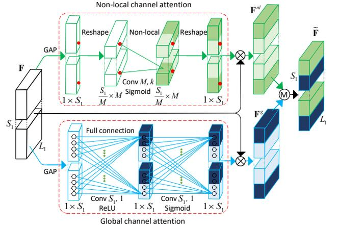
Fig. 5. Diagram of the proposed dual-channel attention. GAP is the global average pooling.  $\otimes$  denotes the element-wise product.  $\textcircled{M}$  illustrates the element-wise maximum.
