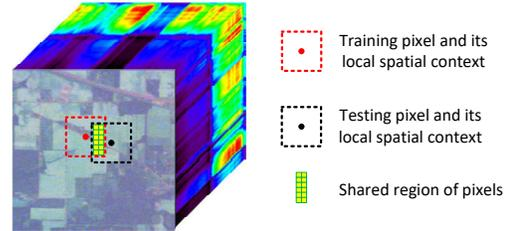
Fig. 1. An illustration of pixel-sharing between the training and testing data. The shared pixels aggravate with a larger window scale or more training data.
