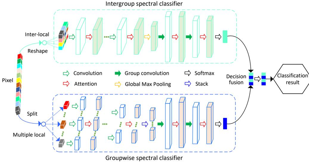
Fig. 2. The overall architecture of the proposed method. The intergroup spectral classifier extracts interlocal spectral correlation features from a matrix that is reshaped from the input pixel vector. The groupwise spectral classifier extracts discriminative local spectral features from groups of sub-bands.
