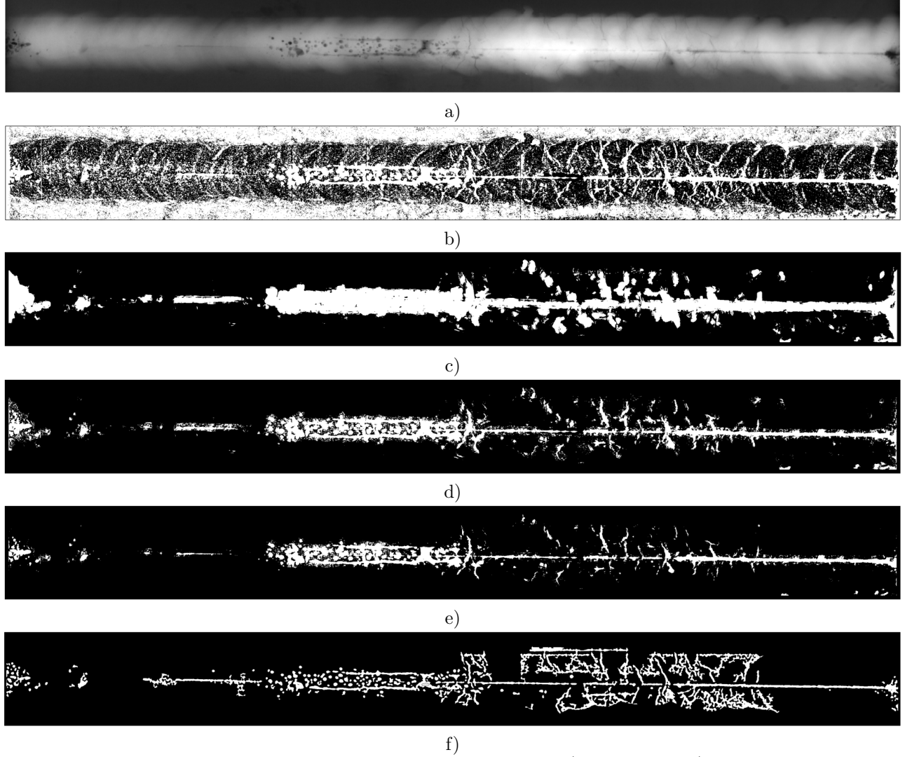
Figure 5. Illustration of the defect detection process for the first test image: a) source image, b) thresholded morphological image, c) Conv.Net, d) Conv.Net + morphological filtering (MF), e) Conv.Net + morphological filtering + enhanced boundaries, f) ground truth defect map
