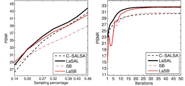
Fig. 3. Left: PSNR values of the reconstructed sagittal MRI slice using radial sampling trajectories with different sampling rates. Right: Reconstruction performances on the same image with 20% of measurements with radial trajectory.
