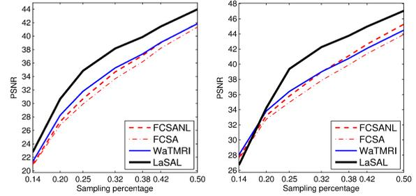
Fig. 4. PSNR values of the reconstructed sagittal MRI slice (left) and the ‘MRI-brain’ image (right) using random sampling trajectories with different sampling rates.
