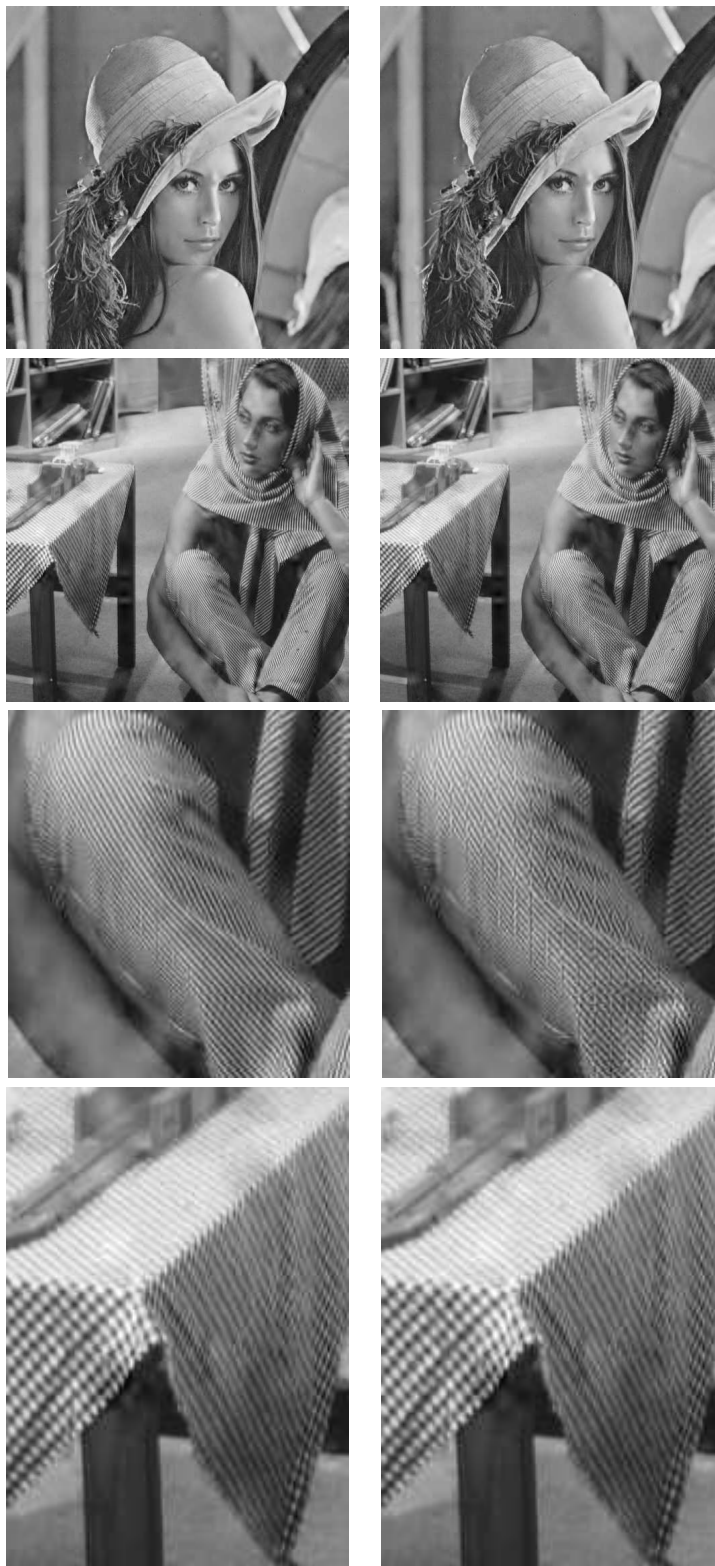
Fig. 8. Performance comparison between the proposed method and its simplified fast version. Left: the full version of the proposed method (The PSNR of Lena and Barbara is 32.14 and 28.27 dB respectively). Right: its fast version (The PSNR of Lena and Barbara is 32.08 and 27.25 dB respectively).
