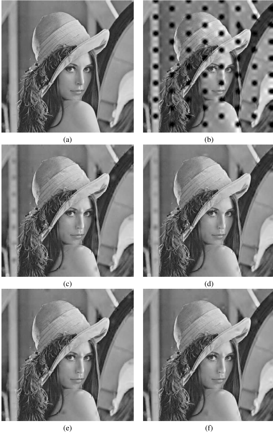
Fig. 5. (a) Lena compressed at 0.8 bpp (PSNR = 38.29 dB). (b) Lena after loss of packet 4. (c) Reconstruction with the bilinear interpolation (PSNR = 30.59 dB). (d) Reconstruction with the adaptive MAP approach of [6] (PSNR = 30.95 dB). (e) Reconstruction with the adaptive method of [7] (PSNR = 31.63 dB). (f) Reconstruction with the proposed method (PSNR = 32.14 dB).
