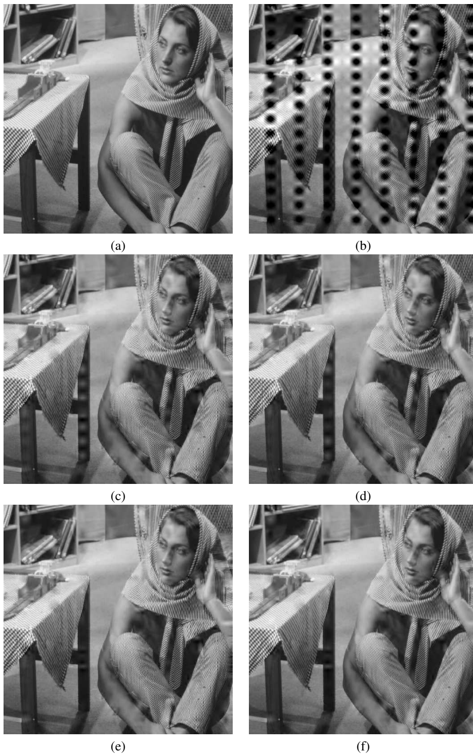
Fig. 6. (a) Barbara compressed at 2.0 bpp (PSNR = 40.54 dB). (b) Barbara after loss of packets 4 and 12. (c) Reconstruction with the bilinear interpolation (PSNR = 26.08 dB). (d) Reconstruction with the adaptive MAP approach of [6] (PSNR = 26.22 dB). (e) Reconstruction with the adaptive method of [7] (PSNR = 26.60 dB). (f) Reconstruction with the proposed method (PSNR = 28.27 dB).
