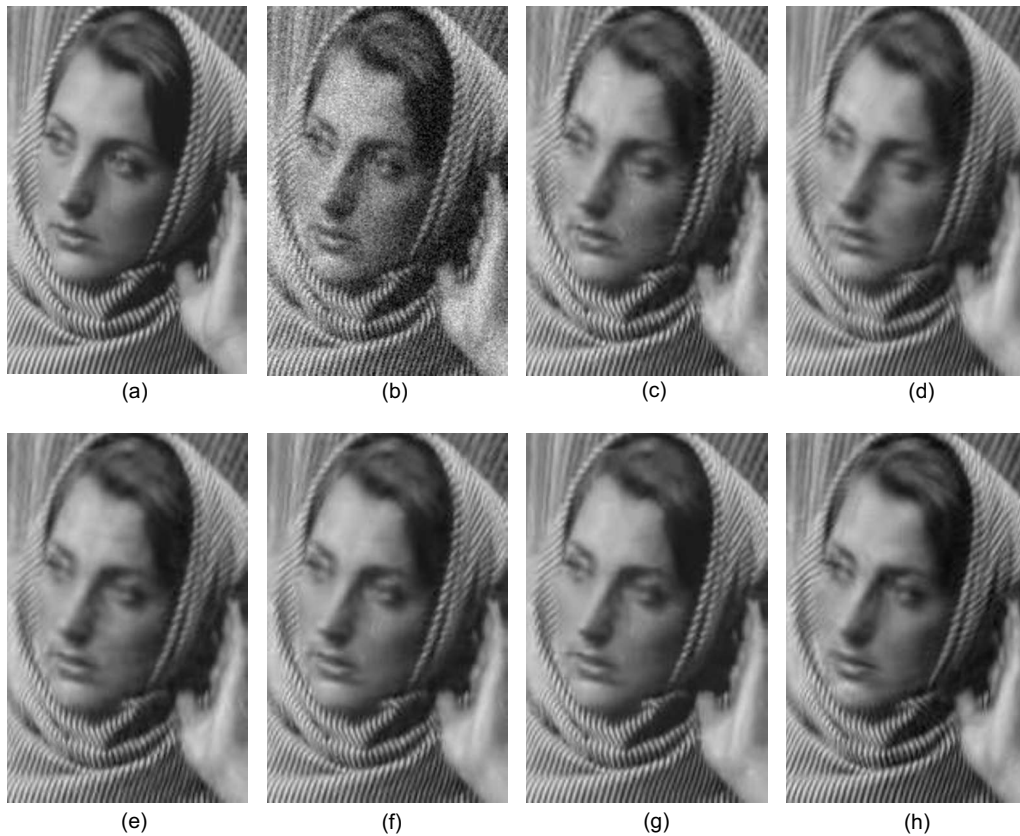
Fig. 9 Details of image Barbara : (a) original image, (b) noisy image (noise standard deviation 20), plus the denoising results of (c) ProbShrink, (d) curvelet hard thresholding, (e) BiShrink, (f) BLS-GSM, (g) BM3D, and (h) ProbShrinkCurv.
