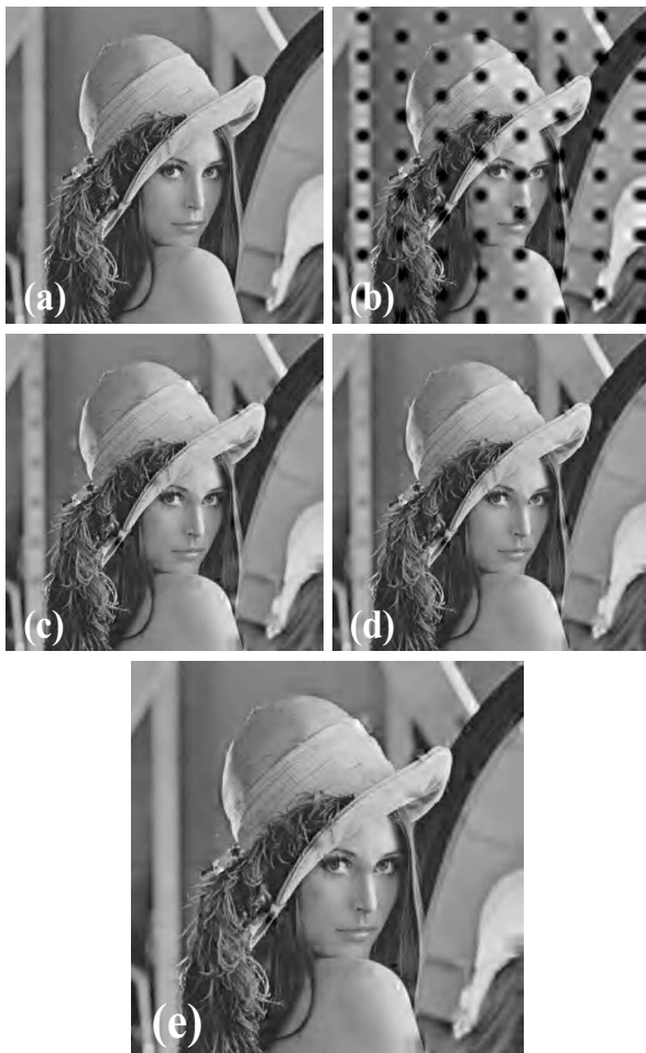
Fig. 2. (a) The Lena -image compressed at 0.21 bpp (PSNR = 32.18 dB). (b) Lena -image after loss of packet 8. (c) Bilinear interpolation (PSNR = 28.35 dB). (d) Adaptive MAP approach [4] (PSNR = 28.92 dB). (e) The proposed method (PSNR = 28.86 dB).
