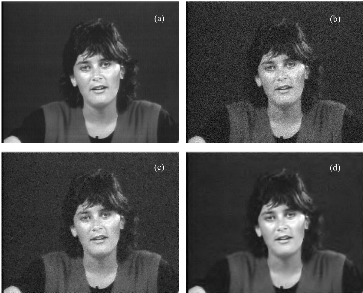
Figure 5. (a) A noise-free frame of the Miss America sequence. (b) Noisy frame, \sigma = 15 . (c) The result of the spatio-temporal filter from [5]. (d) The result of the proposed seqwt-sas filter.
