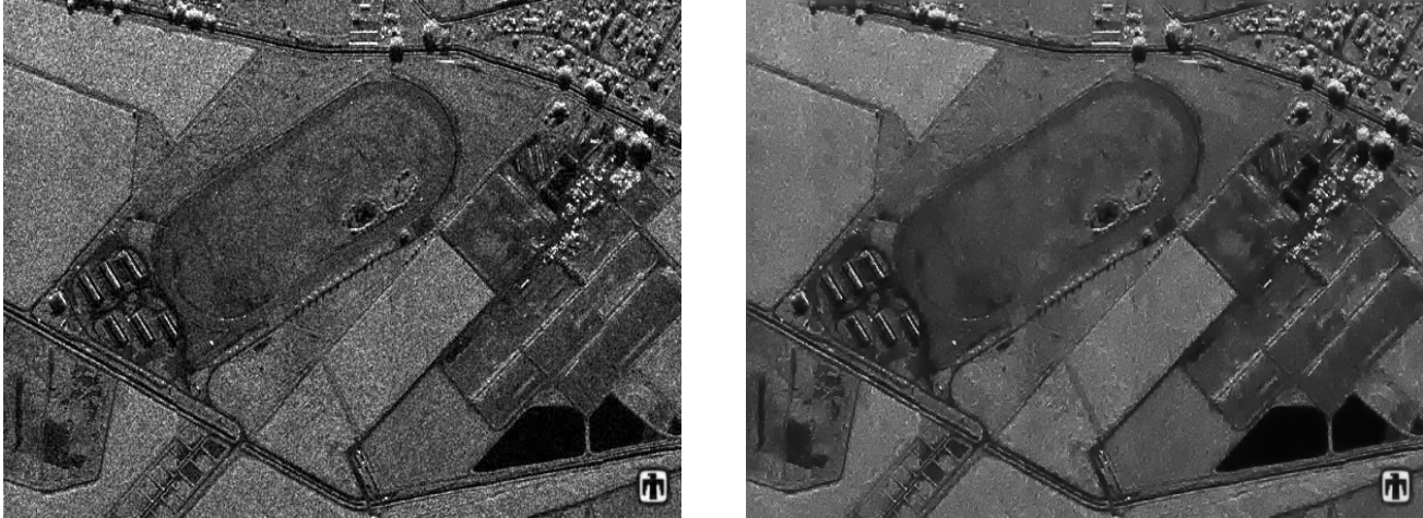
Fig.3. Left: original SAR image showing a horse track, resolution 1m, source Sandia National Lab. Right: Despeckled image.
